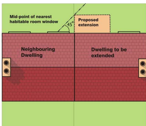
Diagram 5: The '45-degree Rule' applied to a semi detached or terraced property
