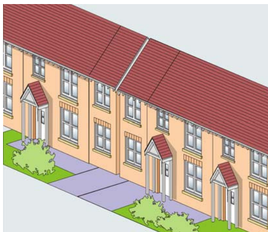
Diagram 11: Inappropriate side extensions which have lead to a 'terracing effect'
